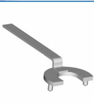
FERRAMENTA PARA TRAVAR A POLIA DA ÁRVORE DE MANIVELAS DO MOTOR EA-111 (II) DO GOL POWER 1.0 16V.
